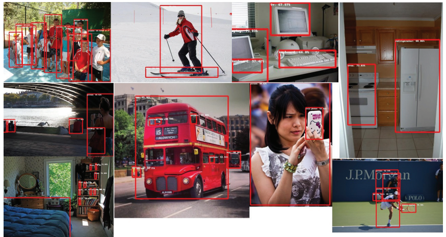
Figure 12. Good inference results. The squares correctly locate object positions and object labels correctly identify object classes.
