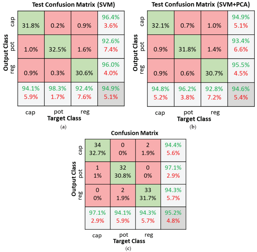
Figure 14. SVM classifiers with cubic kernel function confusion matrices. (a) SVM dataset test; (b) SVM + PCA with 20 components dataset test; (c) Real world test with 104 new objects.
