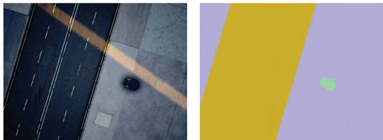
Figure 5. Low-altitude urban scene captured with a downward-looking camera. On the left is a simulated image. On the right is the corresponding segmented scene.
