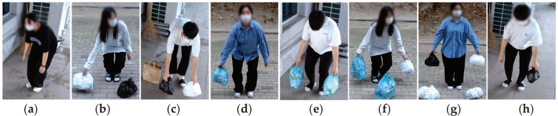
Figure 5. Eight types of scenarios (S1–S8) for the performance evaluation of the illegal dumping monitoring system; (a) S1—a bending posture with no garbage bag; (b) S2—a dumping scenario with the non-standard bag in one hand; (c) S3—a dumping position with the non-standard garbage bags on both hands; (d) S4—a dumping posture with the legal standard garbage bag in hand; (e) S5—a dumping scenario with legal standard garbage bags in both hands; (f) S6—a dumping posture with the standard bag in one hand and the non-standard bag in the other hand; (g) S7—a dumping posture without bending the waist with the non-standard bags in both hands; and (h) S8—a bending position without dumping with the non-standard bag.
