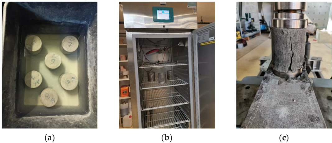
Figure 9. Testing of resistance to freezing and thawing: (a) two-day cure of samples under water; (b) climate chamber; (c) compressive strength test after freezing/thawing cycles.
