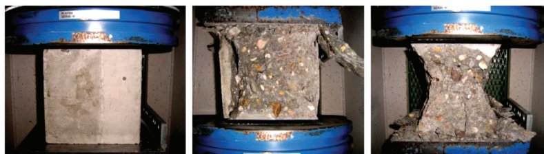
Figure 2. Stages of destruction of the concrete sample during the compressive strength test.
