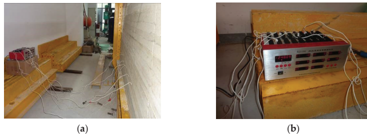
Figure 4. Test systems of two models. (a) Embedded pressure sensor. (b) Static resistance strain gauge.
