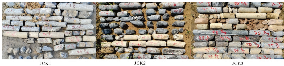
Figure 11. Photos of the cores from the verification boreholes.
