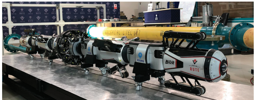
Figure 1. The natural gas inspection robot.
