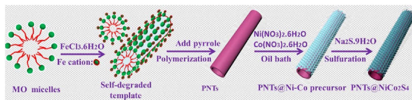
Figure 15. Schematic illustration of polypyrrole nanotubes@NiCo 2 S 4 core-shell formation. Reproduced with permission from Jun Zhang, Hierarchical polypyrrole nanotubes@NiCo 2 S 4 nanosheets core-shell composites with improved electrochemical performance as supercapacitors; published by Elsevier, 2017 [144].
