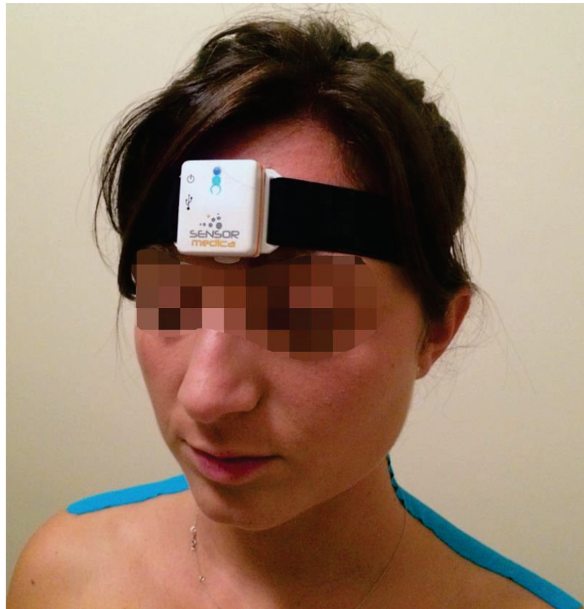
Figure 2. Placement of the inertial sensor on the forehead for measuring of the multiplanar ACROM.
