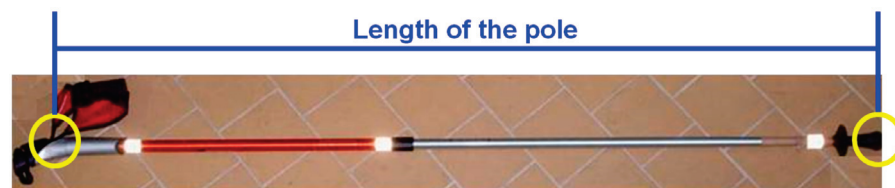
Figure 2. Landmarks for measurement of NW pole's length, from left to right: insertion of the lace in the handle and tip final extremity.
