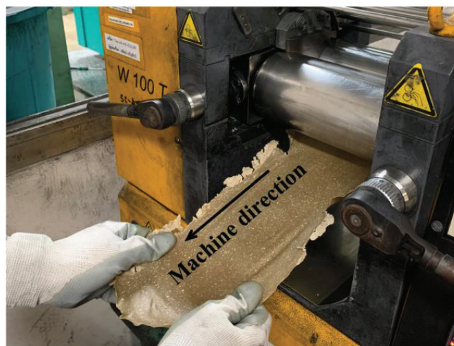
Figure 2. Fiber alignment on a two-roll mill during the uniaxial composite prepreg preparation.
