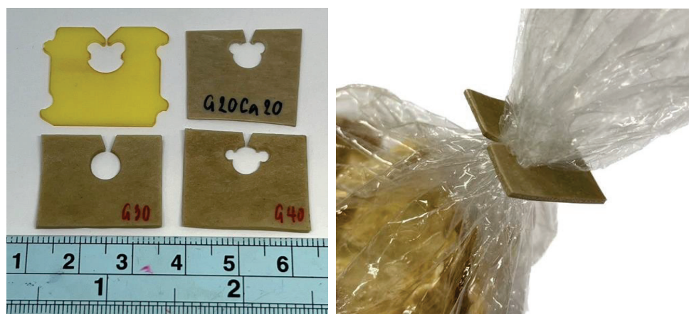
Figure 12. Photographs of simple bread clips made from PSS composites compared with a commercial clip (left) and its use for closing a plastic bag (right).
