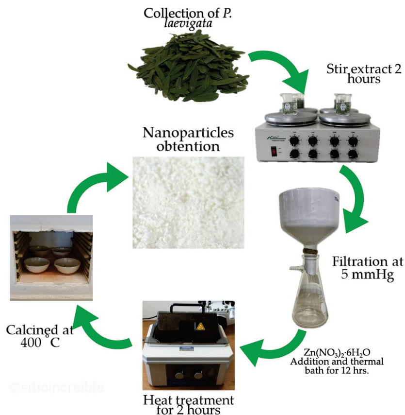
Figure 1. Green synthesis process of ZnO nanoparticles using Prosopis laevigata extract.
