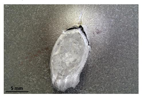
**Figure 14.** Partial penetration of FMJ bullet material through the first plate of Durostat<sup>®</sup> 400. Back of the first plate showing the penetration of some melted filler material.
