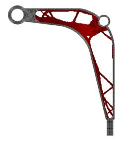
Figure 23. The final topology found for the control arm.
