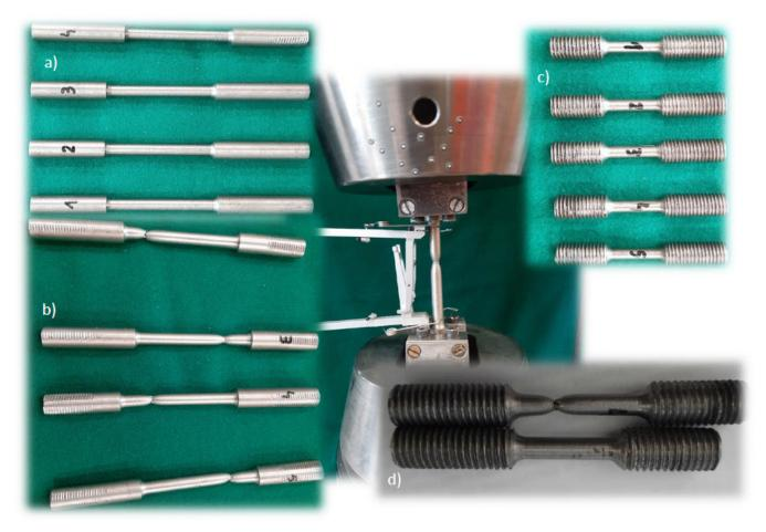
**Figure 3.** HY 80 steel specimens for static and dynamic tests: (**a**) samples for static tests on the MTS machine; (**b**) samples for static tests after fracture; (**c**) samples for dynamic tests on a rotary hammer; (**d**) samples for dynamic tests after fracture.
