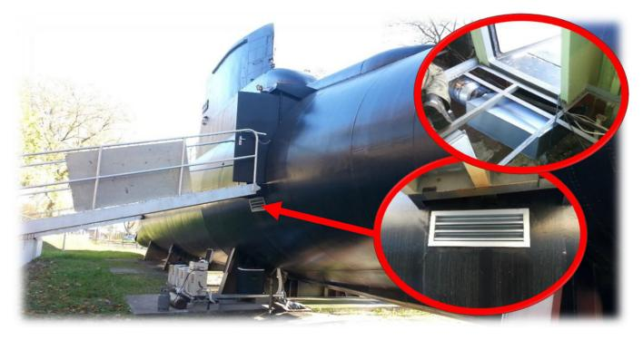
Figure 2. ORP "Jastrząb" (S-318 Kobben). Places from which material was taken for test samples.
