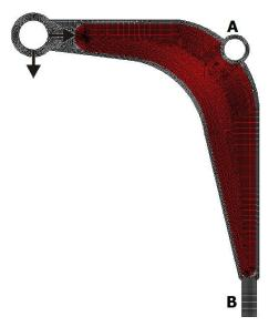
Figure 22. The design domain, loads, and supports of the control arm.
