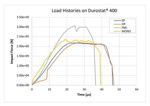
**Figure 17.** Load histories estimated according to Equation (8), applied to the impacts on Durostat<sup>®</sup> 400. The SP, HP and MONO bullets have similar force peaks around 220–230 kN. The FMJ reaches instead 307 kN force. The duration of the impulses ranges from 36 to 47 µs.
