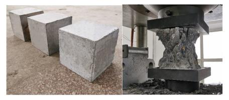
Figure 3. Concrete cubes and the failure mode of concrete tubes.
