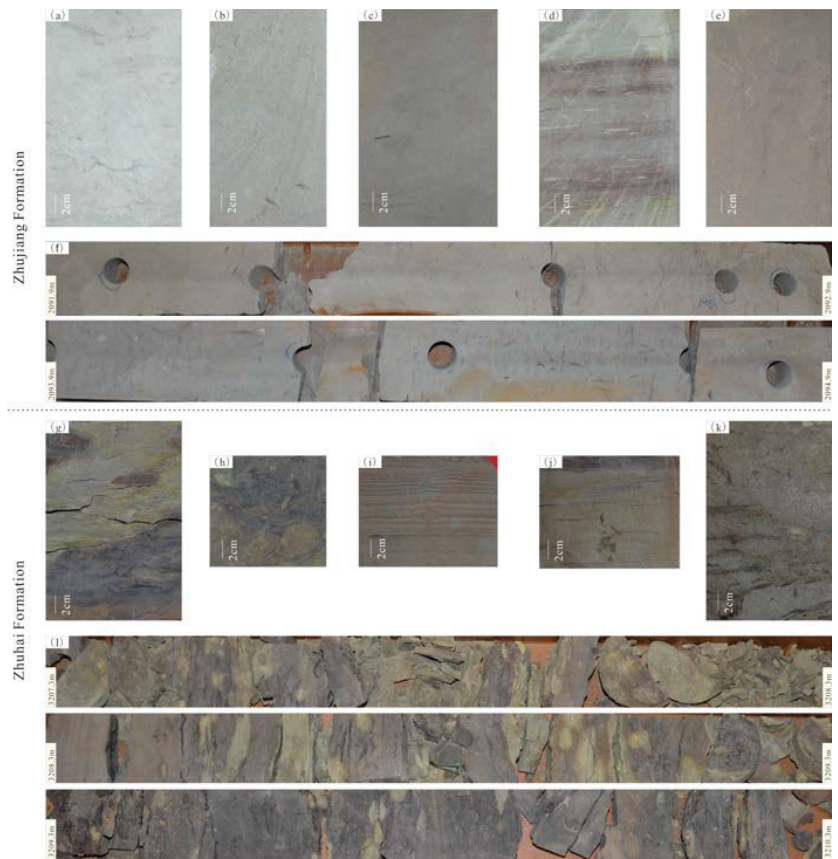
Figure 5. Typical sedimentary characteristics of the deposits in the Zhujiang (a–f) and Zhuhai (g–l) Formations in the Zhu III Depression: (a) 2092.5 m in Well W4, siltstone; (b) 2092.8 m in Well W4, siltstone; (c) 2090.2 m in Well W4, fine-grained sandstone; (d) 2091.3 m in Well W4, fine-grained sandstone and siltstone with parallel bedding; (e) 1220.3 m in Well W32, fine-grained sandstone with normally graded bedding; (f) 2.0 m (2091.9–2092.9 m and 2093.9–2094.9 m) long core of the shallow-marine detrital deposits from the Zhujiang Formation; (g) 3210.7 m in Well W3, siltstone interbedded with mudstone; (h) 3210.9 m in Well W3, siltstone interbedded with mudstone; (i) 1861.2 m in Well A3, tidal rhythmites; (j) 1816.4 m in Well A3, tidal rhythmites; (k) 3211.1 m in Well W3, fine-grained sandstone interbedded with mudstone; (l) 3.0 m (3207.3–3210.3 m) long core of the tidal flat deposits in the Zhuhai Formation.
