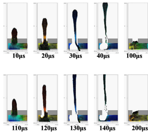
Figure 5. Calculate and simulate water in a single-channel jet cavity with a nozzle diameter of 60 μm and a thickness of 50 μm, with an operating frequency of 10 KHz, in the XZ two-dimensional cross-sectional view, at 10, 20, 30, 40, 100, 110, 120, 130, 140 and 200 μs injection situation.
