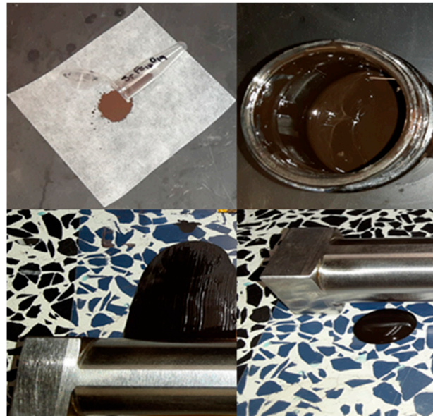
Figure 2. As synthesized strontium ferrite nanopowder, formulated ferrite paste and ferrite paste before and after spreading by doctor blade onto a plastic substrate.
