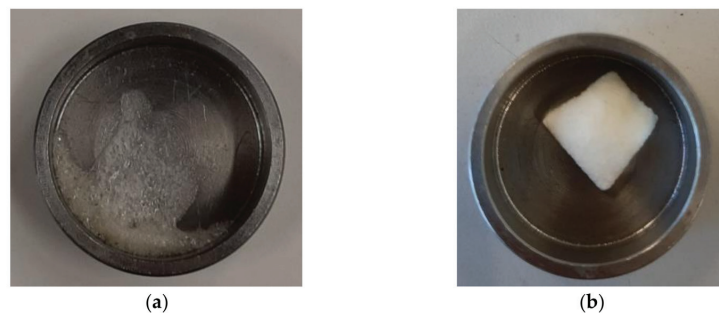
Figure 5. Macroscopic structure of electrospun PCL films after contact with scCO 2 : (a) not optimized and (b) optimized.
