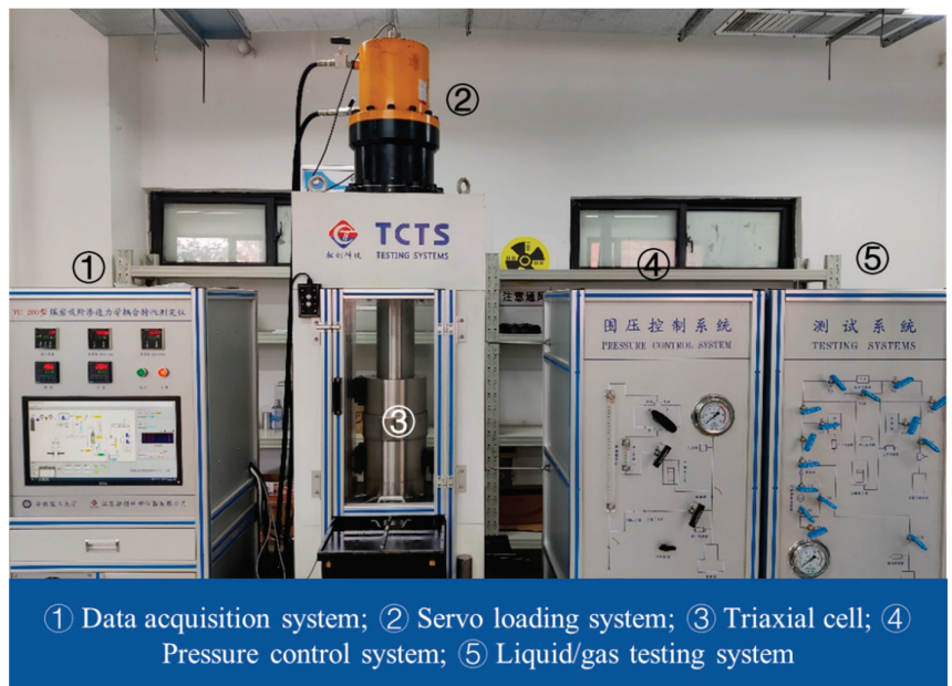
Figure 2. Triaxial servo-controlled mechanical-seepage coupling experimental apparatus [29].
