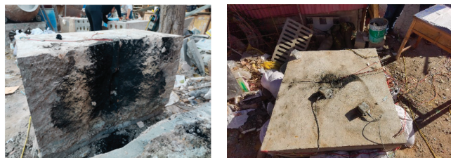
Figure 5. The test block after blasting.
