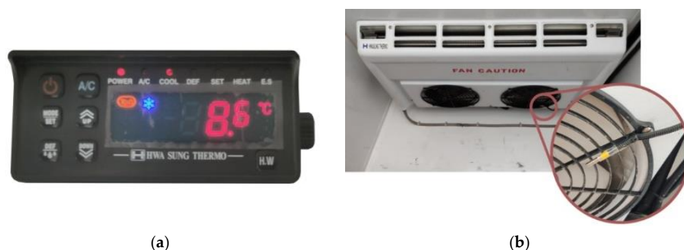
Figure 4. Controller (a) and heat exchanger with temperature sensor (b) of the trucks refrigeration system.
