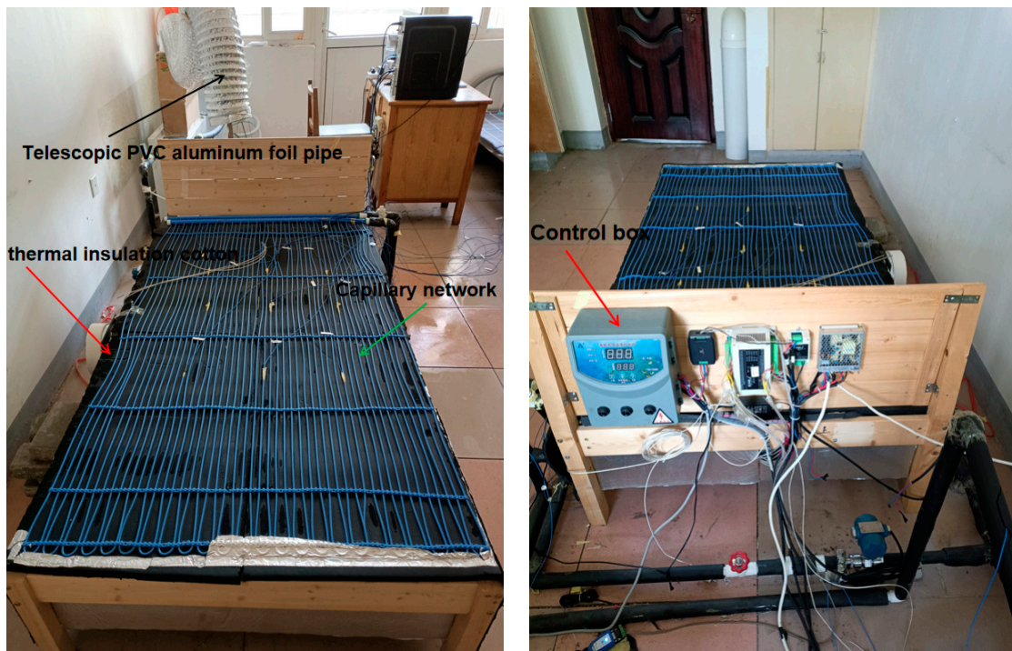
Figure 2. Physical diagram of capillary convection and heat conduction air-conditioned bed system.
