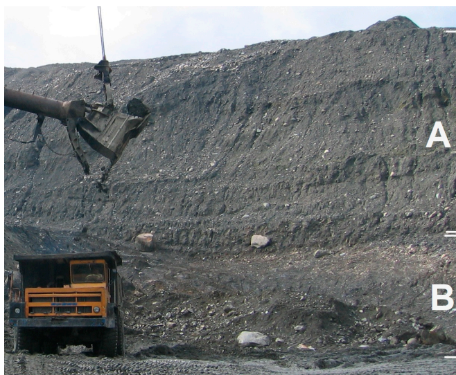
Figure 7. Cross-section of deposits of the placer of R. Nygri. (A) man-made tailing dumps; (B) the deposits of the second stage.
