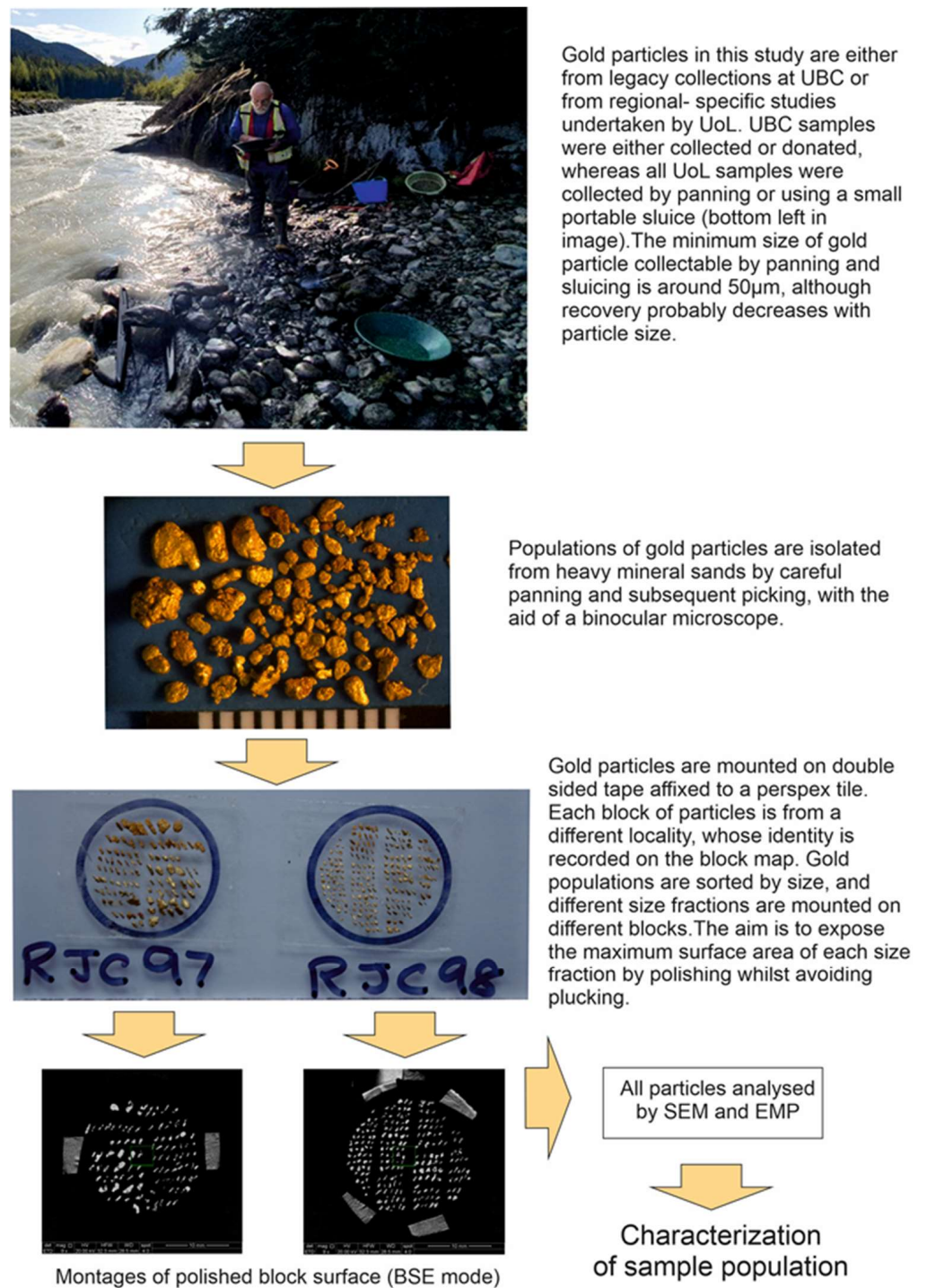
Figure 2. Schematic representation of the project workflow for the collection and characterization of gold particles.
