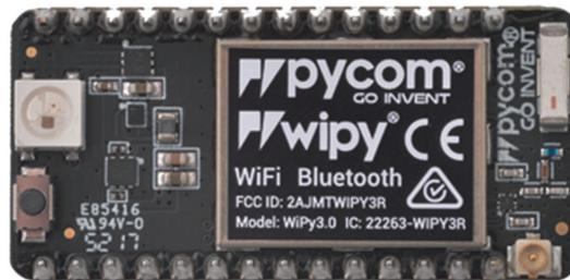
Figure 2. WiPy 3.0 development board based on ESP32 chip.
