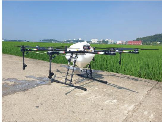
**Figure 2.** Agricultural spraying drone with quad rotor (SG-10P).
