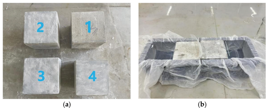
Figure 7. Sample preparation: (a) experimentally prepared hydrophilic coating specimen, hydrophobic coating specimen, superhydrophobic coating specimen; (b) ice adhesion strength test sample making mold diagram.
