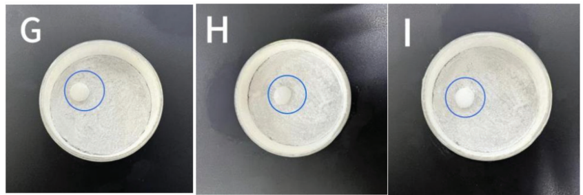
Figure 6. After the water droplets freeze on the sample surface. (A–C) Photos of droplets freezing on the surface of the regular specimen; (D–F) photos of drops of water on the surface of the hydrophobic coating specimen; (G–I) photos of droplets on the surface of the superhydrophobic coating specimen.
