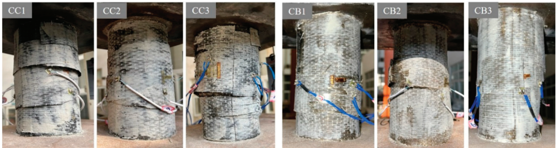
Figure 6. Pictures of the composite columns after destruction.
