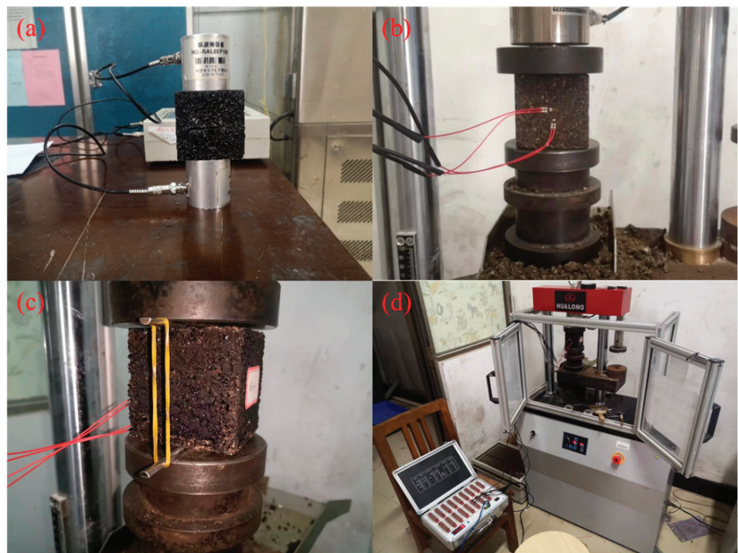
Figure 4. Test procedures: (a) ultrasonic pulse velocity; (b) UCS test; (c) ITS test; and (d) static creep test.
