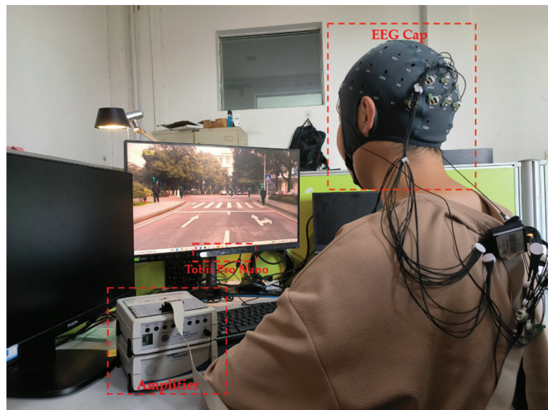
Figure 3. Placement of data acquisition equipment.
