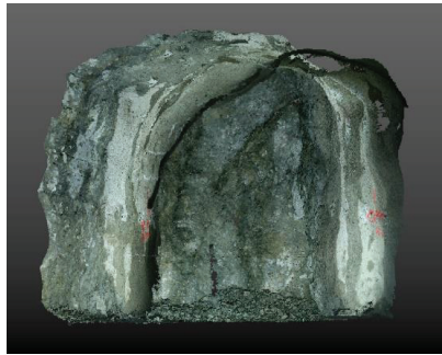
Figure 3. Typical drift environment point cloud data by SLAM.
