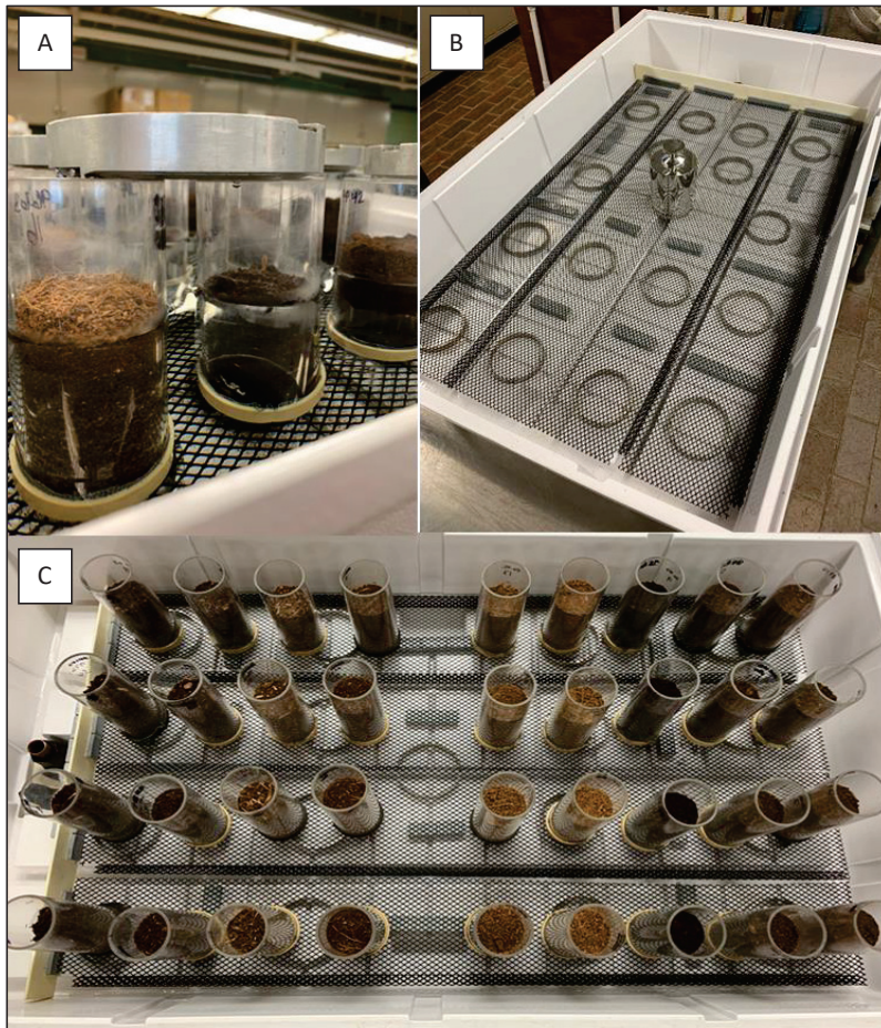
Figure 3. Ebb and flood subirrigation system. (A) Container capacity testing with 2 kg aluminum weights. (B) Partially constructed ebb and flood unit with aluminum rings with mesh screen. (C) Fully constructed system complete with packed substrate cylinders.
