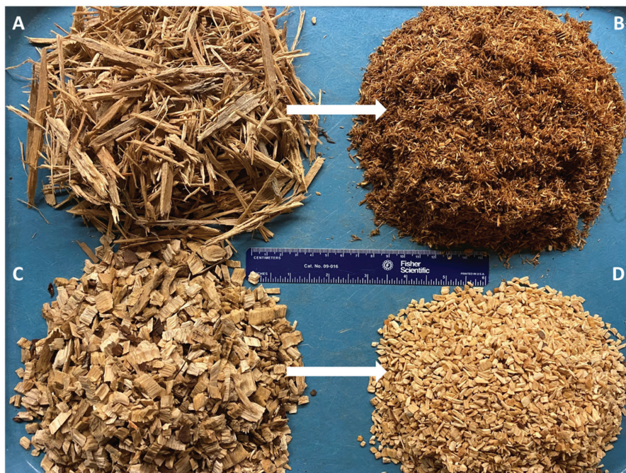
Figure 2. Pre and post hammer mill processing on the shredded pine wood (SPW) and pine wood chips (PWC). Shredded wood (A) passed through the hammer mill to produce SPW (B). Chipped pine wood (C) is passed through a hammer mill to produce PWC (D).
