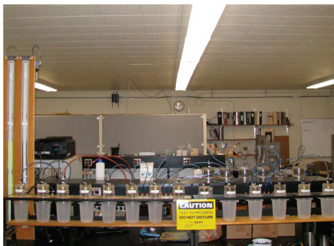
Figure 2. Setup of the Tempe cell experiment.
