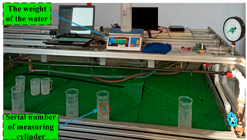
Figure 4. Drip irrigation emitters flow test platform.
