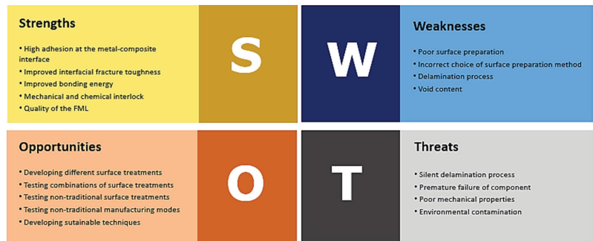
Figure 16. SWOT analysis showing the impact of surface treatment on the adhesion of dissimilar materials during the production of FML stacks.
