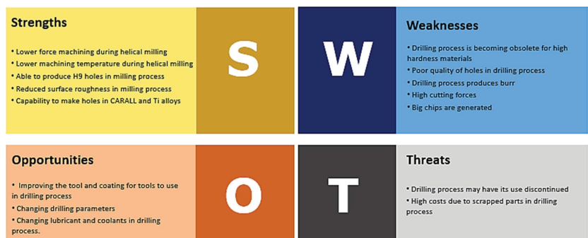
Figure 17. SWOT analysis obtained by comparing between drilling and milling processes in FML.
