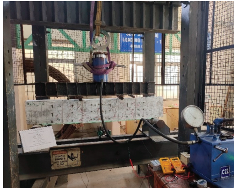
Figure 3. Test setup of the beam with smart mortar layer.
