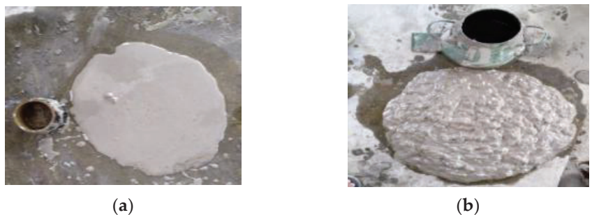
Figure 2. Workability test on ECC. (a) Mini-slump test; (b) standard slump test.
