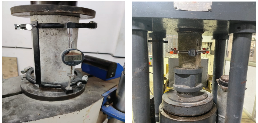
Figure 8. Compressometer test for lateral strain and linear strain measurements.
