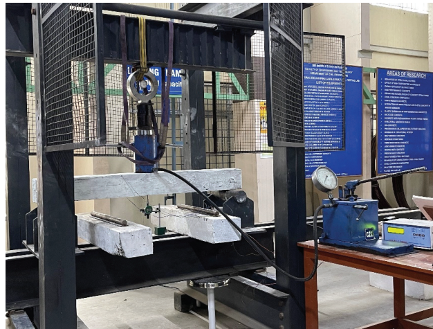
Figure 9. Experimental setup for testing of beam.
