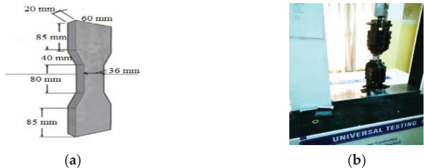
Figure 3. Direct tensile strength test setup. (a) Dog-bone-shaped specimen; (b) direct tensile strength test setup on ECC.
