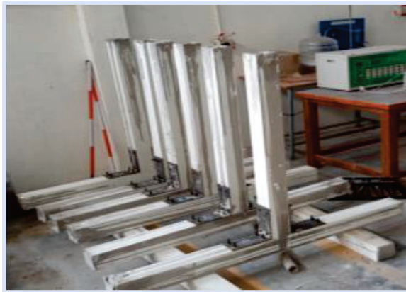
Figure 5. The casting of GFRP beam-column specimens.
