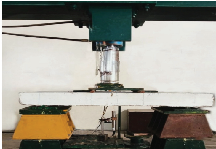
Figure 3. Testing of the slab specimens.
