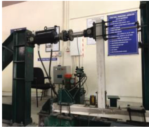
Figure 7. Experimental setup for lateral loading on beam-columns.
