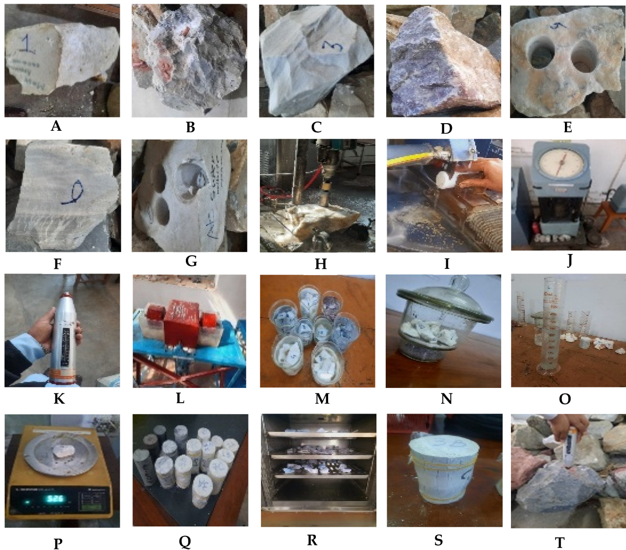
Figure 1. (A) Afghanistan marble, (B) Mardan (spin kala) marble, (C) Chitral marble, (D) Mohmand marble, (E) Bunir Bumpoha, (F) Chitral marble, and (G) Mohmand (super white) marble. (H) Core drilling, (I) core cutting, (J) triaxial testing machine, (K) Schmidt hammer apparatus, (L) slake durability apparatus, (M) sample dipped for 24 h, (N) desiccator used to cool sample, (O) volumetric cylinder used to find volume, (P) sampling weight, (Q) core samples, (R) oven for drying samples, (S) core failure after UCS testing, and (T) sampling using a Schmidt hammer.
