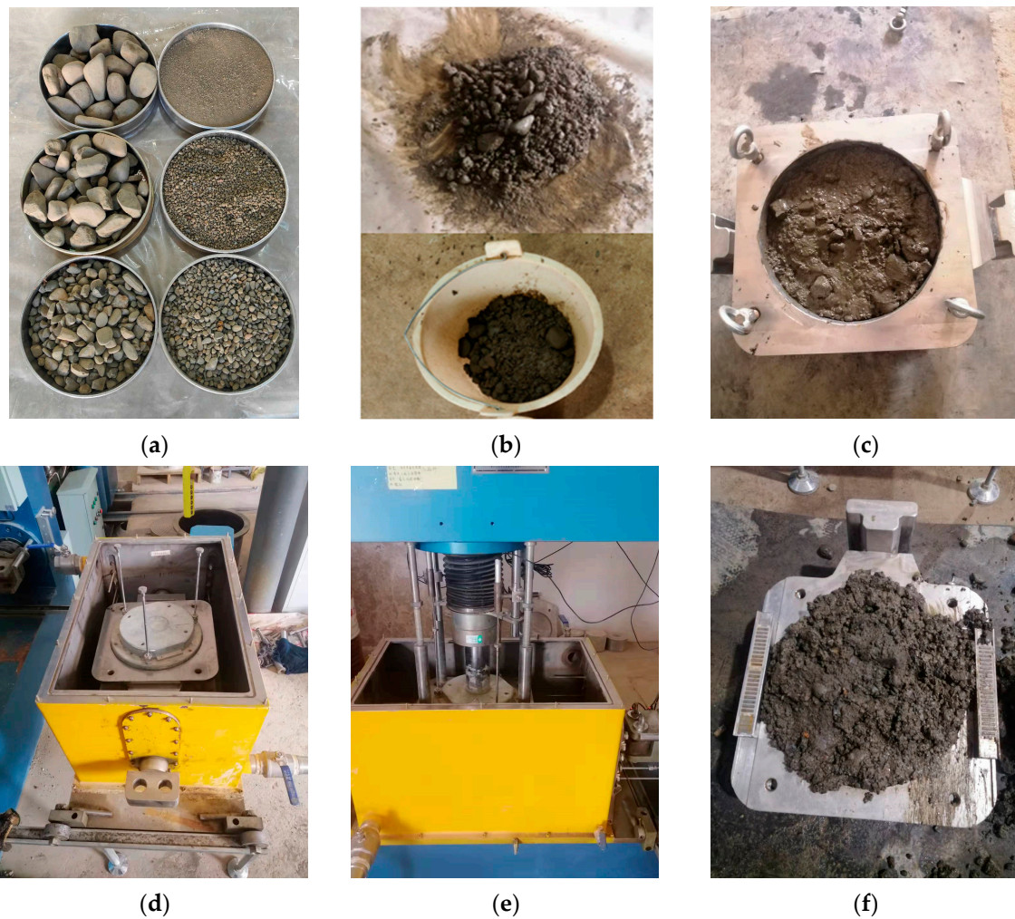
Figure 5. Experimental steps for direct shear of round gravel soil: (a) sieving soil; (b) soil mixing and enclosing; (c) load soil sample into shear box; (d) lift the shear box into the test chamber; (e) install the sensor and start the experiment; (f) observe the shape of the cutting surface.
