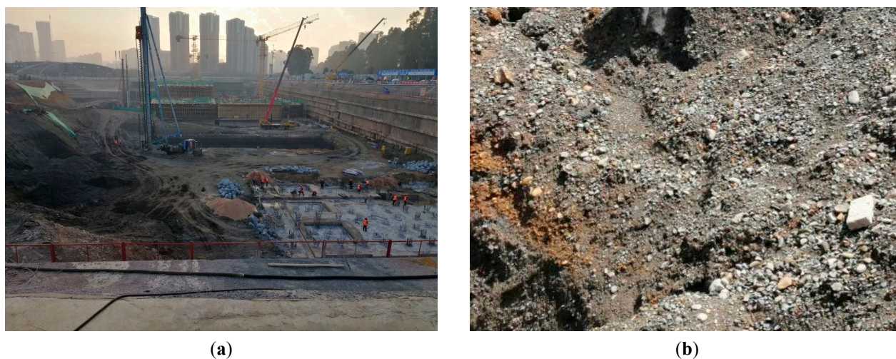
Figure 2. Photos of round gravel soil sampling points: (a) project site photos; (b) photo of sampling point.
