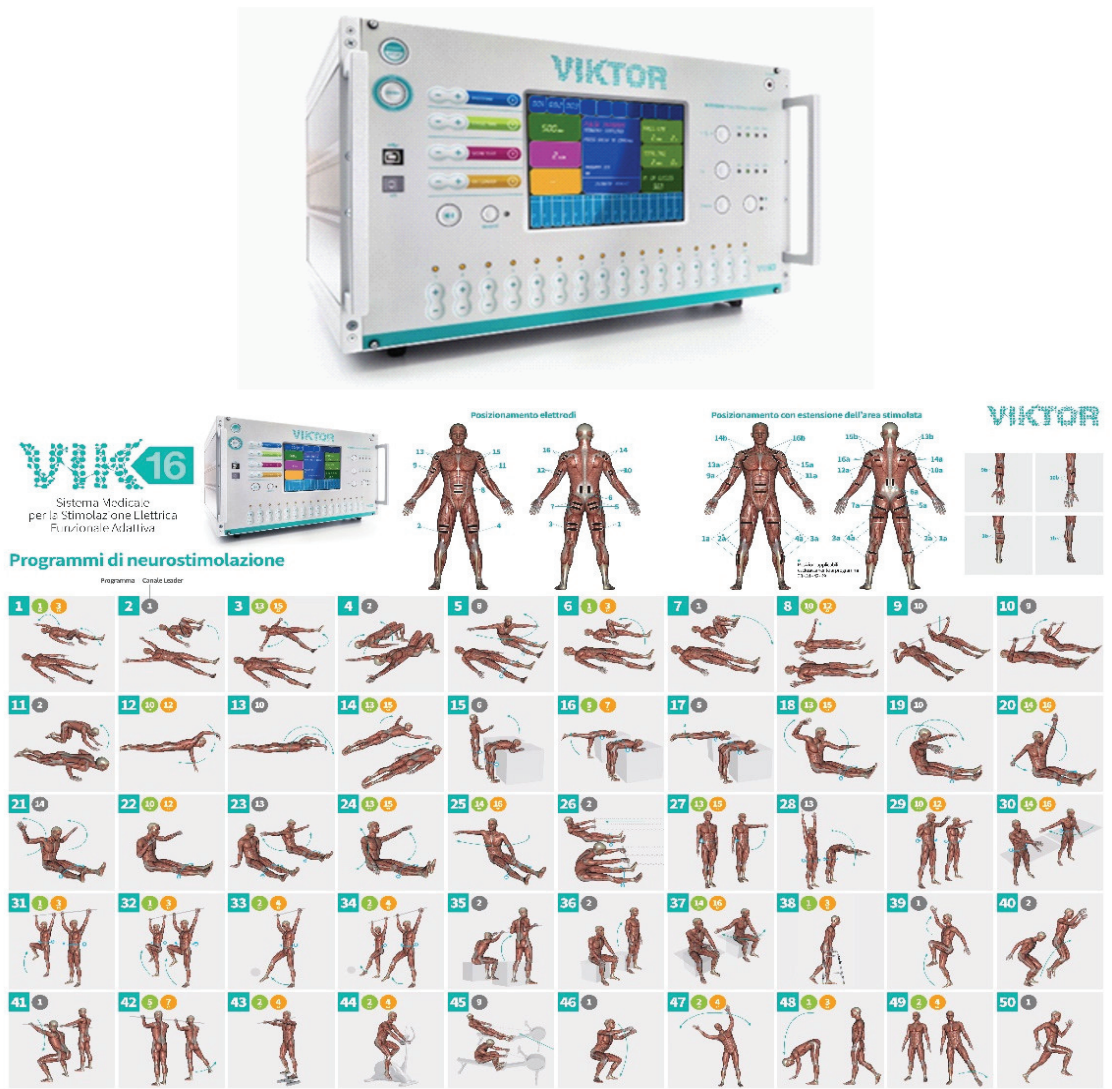
Figure 2. Graphic representation of the VIK16 Workstation and of the set of proposed total-body exercises. Workstation VIK16 has a library of 50 AFESK exercise programs that are used in rehabilitation, athletics and sports training. The programs are created on the basis of polymyographic and biomechanical assessment of the movement of healthy people, considering synergistic, reciprocal and antagonistic relationships of the moments of activation of the main muscle groups of the body. Workstation VIK16 has a wide range of electrical stimulation parameters: including current stabilized in each of 16 channels maximum of 150 mA, duration of a pulse from 100 to 1000 \mu s, pulse frequency from 50 to 200 Hz, motion cycle time from 200 ms to 10 s, impedance parameters and current level for each muscle group for all exercises performed by the patient, customizable number of cycles (movements) for each program and time for each exercise. In this study, only a subset of the exercises was performed by the enrolled patients.
