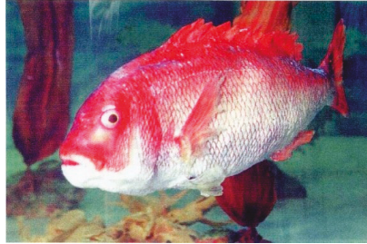
Figure 1. Sea bream robotic fish.
