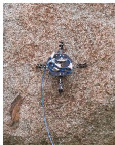
Figure 16. Stably grabbing the rough rock wall.
