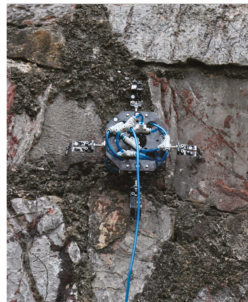
Figure 15. Stably grabbing the granite wall.
