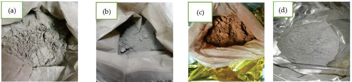
Figure 1. Raw materials were utilized in the preparation of samples: (a) tin, (b) silver, (c) copper, and (d) indium.
