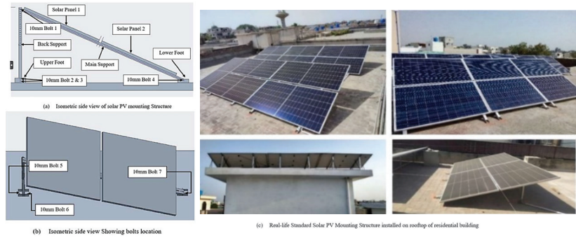
Figure 2. The 14-gauge solar PV mounting structure with 2 solar PV modules.
