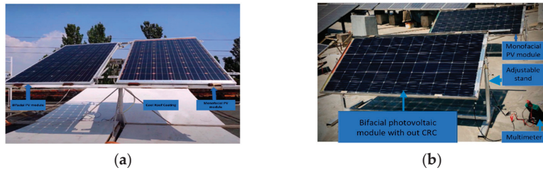
Figure 1. Bifacial and monofacial photovoltaic modules with CRC (a) and bifacial and monofacial photovoltaic modules without CRC (b).
