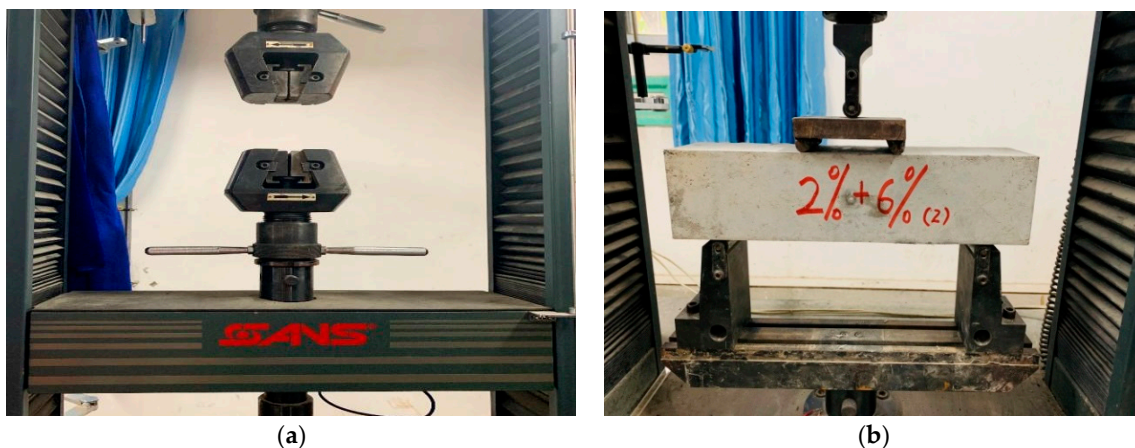
Figure 4. Flexural strength test schemes. (a) Flexural strength test. (b) Flexural strength test specimens.
