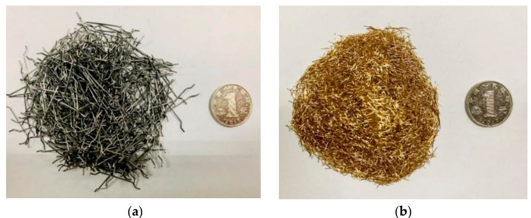
Figure 1. The OS and MS fibers. (a) Ordinary-sized steel fiber (OS). (b) Micro-steel fiber (MS).
