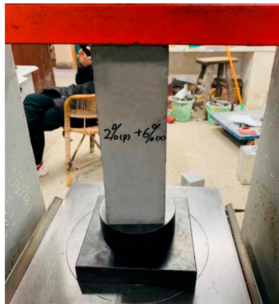
Figure 5. Axial compressive strength test.
