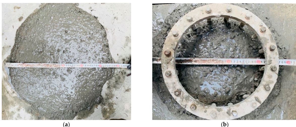
Figure 2. Concrete fluidity test. (a) Slump flow test. (b) J-ring extension.
