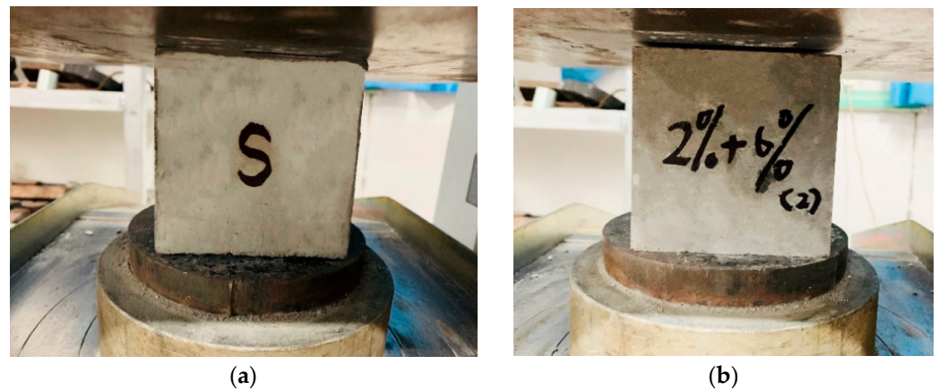
Figure 3. Cube compressive strength test schemes. (a) PSCC. (b) MOSCC-OS1 + MS6.
