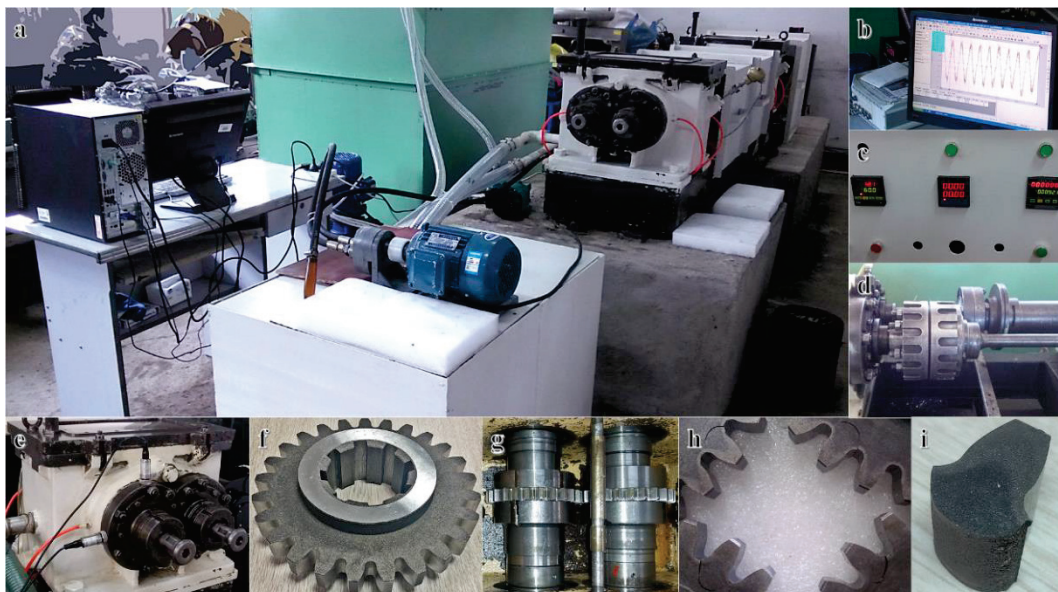
Figure 15. Gear bending fatigue test: (a) test platform; (b) vibration monitoring; (c) revolution counter; (d) loading device; (e) acceleration sensor; (f) gear sample; (g) gear installation; (h) root crack; (i) fracture morphology.
