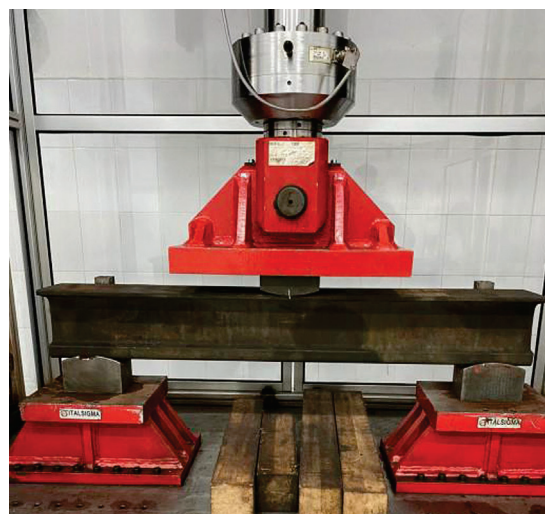
Figure 4. Experimental plant and a general view of tests for determining the endurance limit of the rails.
