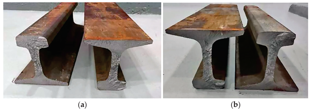
Figure 11. Rail failure after cyclic tests: (a) under a load of 700 kN, number of cycles: 790,056; (b) fracture under a load of 600 kN, number of cycles: 1,111,966.
