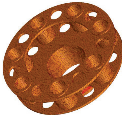
Figure 2. Example of FE model and geometry of planet carrier.
