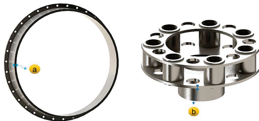
Figure 18. Sensitivity dimensions of system performance indexes: (a) rim thickness of the ring gear (b) base plate thickness of the planet carrier.
