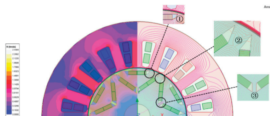
Figure 7. No-load magnetic field distribution cloud map in \nabla shape rotor structure.
