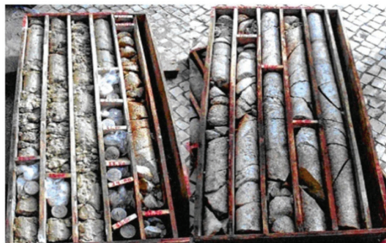
Figure 3. Geological sampling results of the tunnel.
