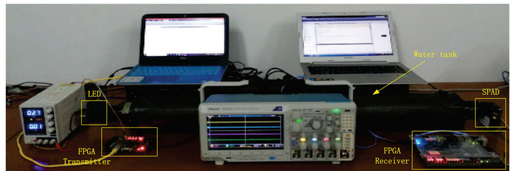
Figure 11. Diagram of the water tank experimental system.
