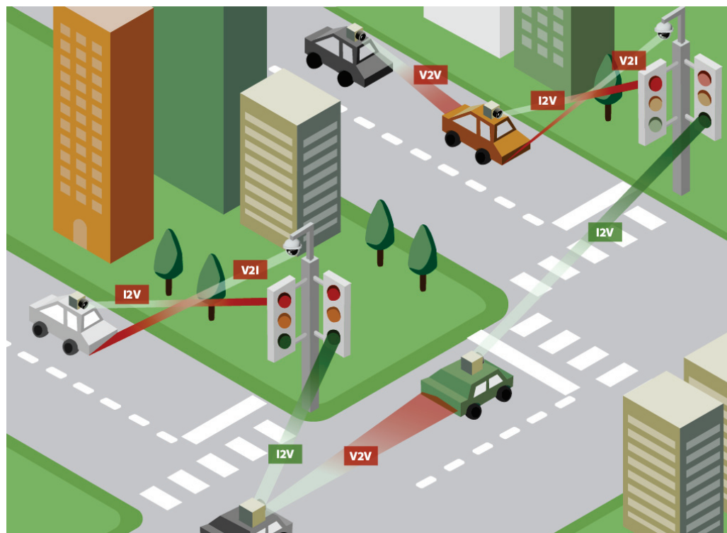
Figure 6. The basic idea of image sensor communication for vehicular applications including vehicle-to-vehicle (V2V), vehicle-to-infrastructure (V2I), and infrastructure-to-vehicle (I2V) communications. Data signals are emitted from traffic lights and vehicle headlights and taillights. Image sensors are mounted on the vehicle to receive visible light signals. The image sensor converts the received visible light signal into an electrical signal and decodes the signal using image processing technology.
