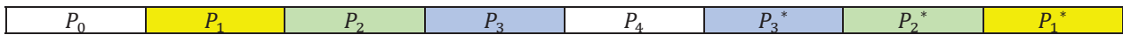
Figure 4. The subcarriers for eight real input samples at the output of the FFT module.
