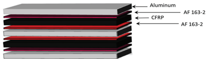
Figure 1. FML layup sequence adopted in this work.
