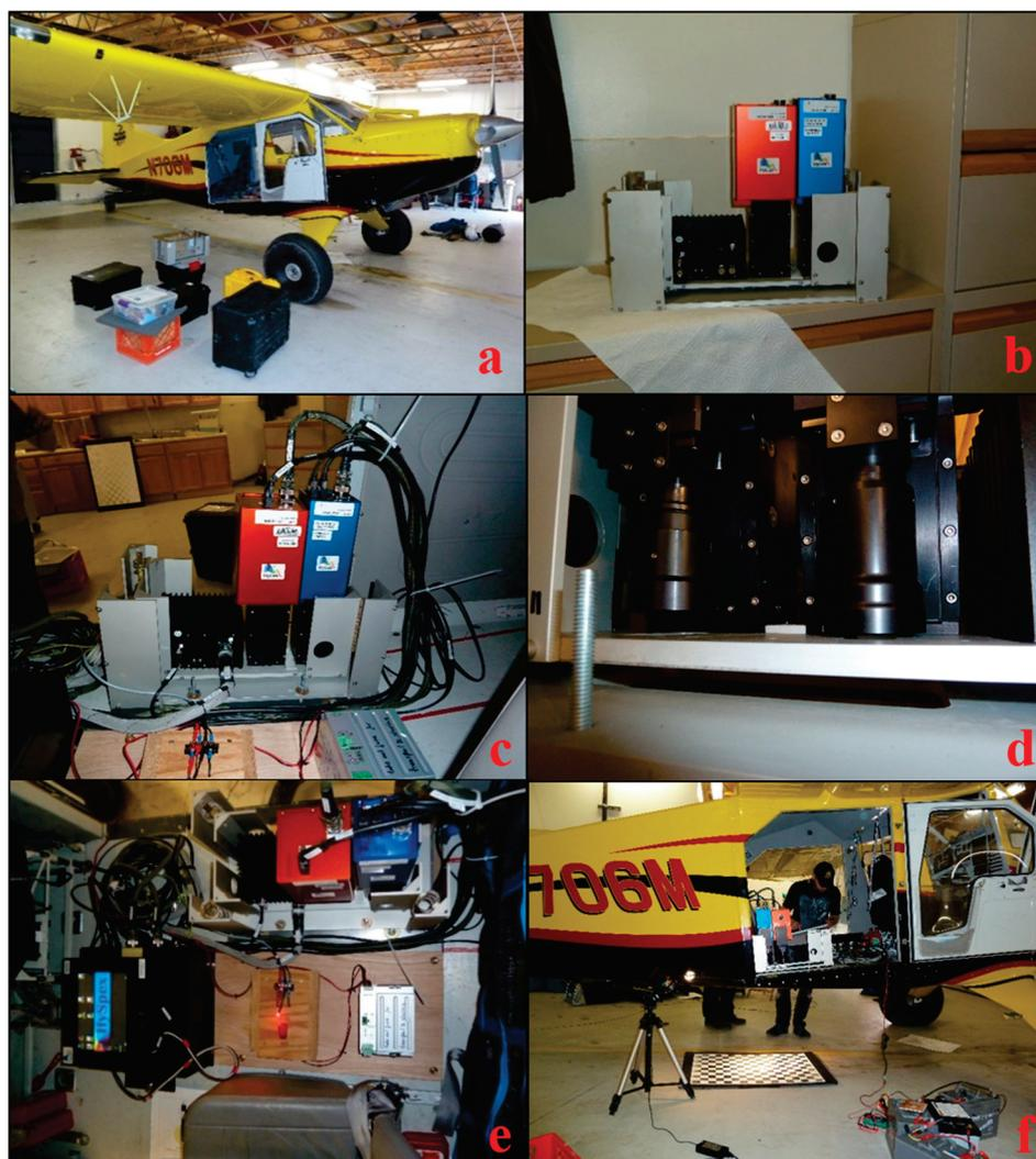
**Figure 2.** Commissioning the HySpex system for airborne acquisition. (a) Refuge Found Bush Hawk; (b) VNIR-1800, SWIR-384, and IMU/GPS units mounted to vibration dampening plate; (c) field of view expander optic attached to VNIR-1800 and SWIR-384 sensors; (d) detail of HySpex sensors in aircraft; (e) overhead view of the system secured and operating in aircraft; (f) testing system visibility through floor aperture of the aircraft.
