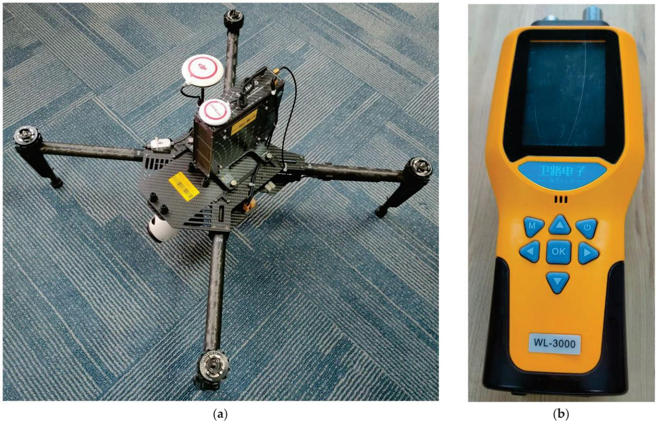
**Figure 2.** (a) UAV-based sniffer4D sensor; and (b) portable gas detector.
