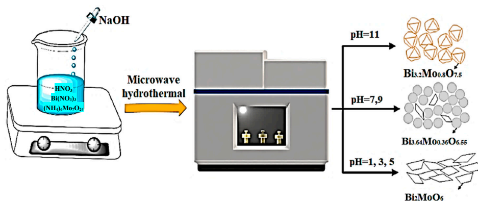
Figure 2. The schematic illustration of the formation of bismuth molybdate catalysts (Reprinted with permission from Ref. [35]).
