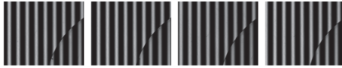
Figure 7. A fringe pattern from the disk experiment and its corresponding phase-shifting fringe patterns.
