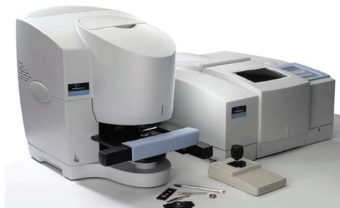
Figure 8. Photo of a commercial Fourier transform infrared (FT-IR) spectrometer equipped with different options for acquisition of spectra in different geometries at micro and macroscopic levels.
