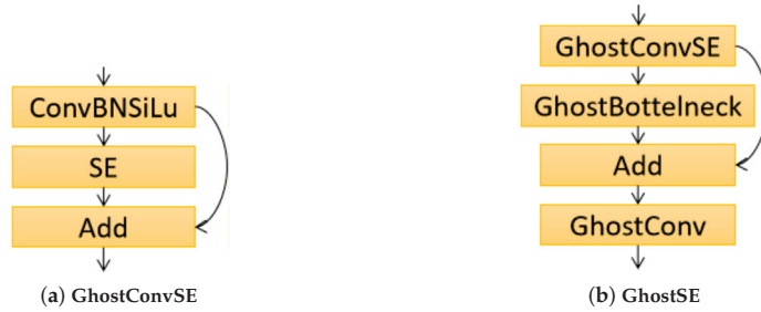
Figure 3. The left image shows GhostConvSE, which uses SE attention to obtain more feature information; the right image shows GhostSE.
