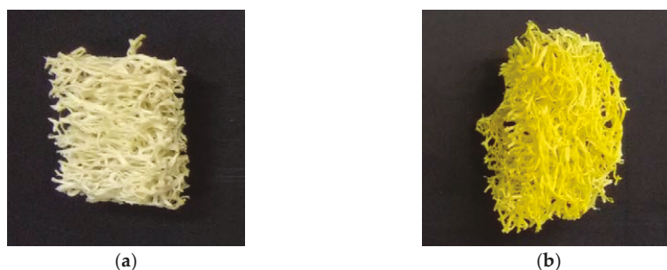
Figure 1. Loofah sponges cubes after total enzymatic activity assay; (a) unimmobilized carrier (b) loofah cubes after incubation with Planococcus sp. S5 cells.
