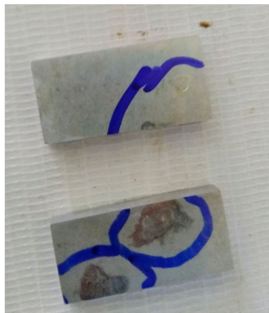
Figure 7. Corroded specimen after immersion test.
