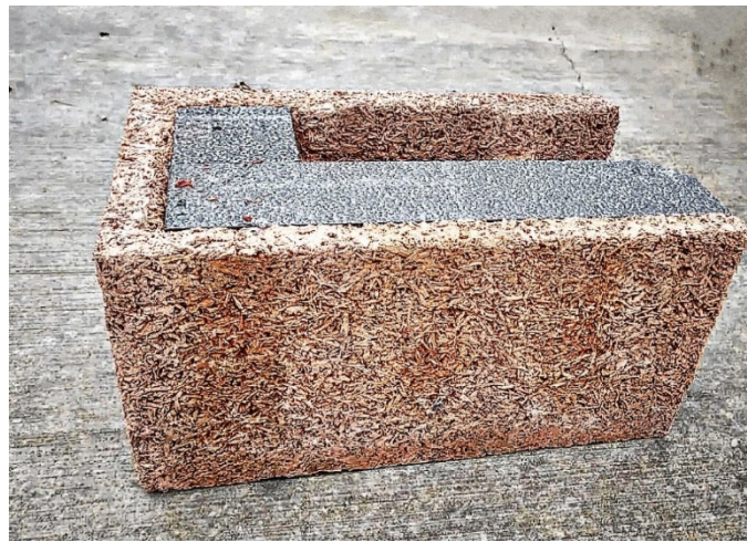
Figure 1. Concrete block with wood chips.
