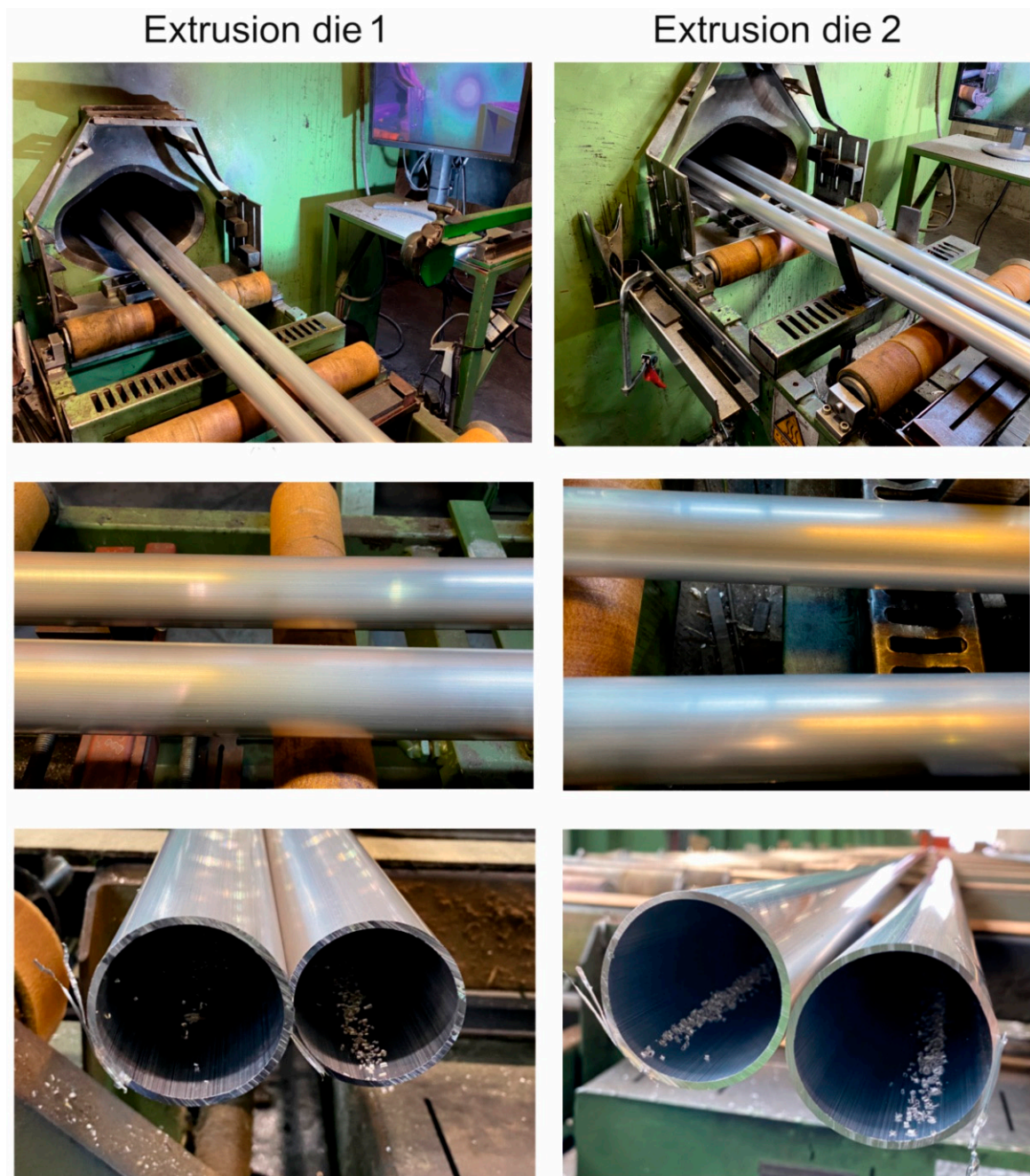
Figure 20. Extruded tubes of \text{Ø}50 \times 2 mm from 7021 alloy 2 on the press run-out for dies of different geometries: die 1; T_0 = 480 °C, V_1 = 3.5 m/min, die 2; T_0 = 480 °C, V_1 = 4.5 m/min.
