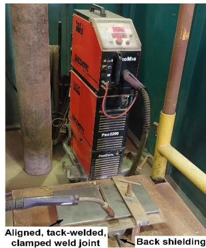
Figure 2. Experimental setup of GMA welding experiments.
