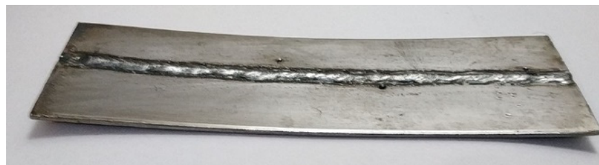
Figure 13. The weld sample for validation.
