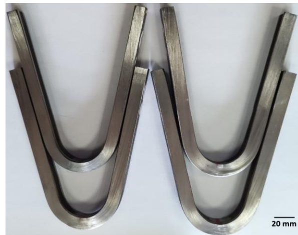
Figure 7. View of the samples after bend test.
