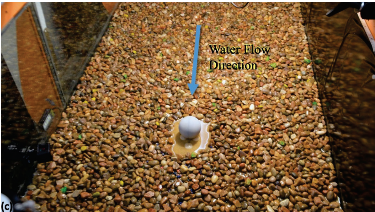
Figure 1. Illustration of the experimental setup: (a) sketch of the side view of the flume, also showing the test section and the relevant instrumentation (acoustic Doppler velocimetry and the instrumented particle), (b) the top view and (c) photo from the experimental setup, illustrating the use of the instrumented particle sitting on top of a dedicated 3D-printed micro-topography, transferring entrainment data in real time via the WiFi protocol (effective for submergence depths below 13.5 cm—see the WiFi antenna attached on the frame above the target particle), the high-speed video camera (used for visually assessing particle entrainments from the side) and the instrumented particle. The flow direction is also shown.
