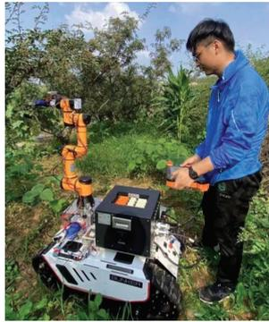
**Figure 10.** Peppercorn-picking robot test platform.
