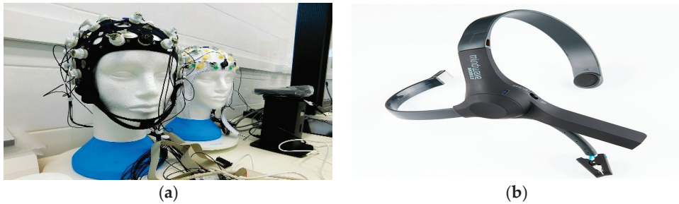
Figure 5. (a) Conventional lab EEG headset [29] versus (b) wearable headset from NeuroSky [30].
