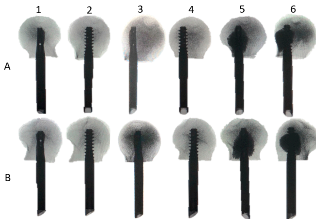
Figure 2. Exemplified samples of each group in superoinferior (A) and anteroposterior (B) views; groups 1 and 2: helical blade and screw in centre–centre position; groups 3 and 4: helical blade and screw in 7 mm anterior off-centre position; groups 5 and 6: helical blade and screw in 7 mm anterior off-centre position augmented with bone cement.
