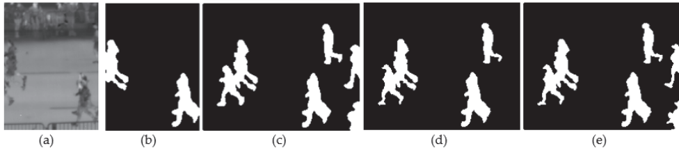
Figure 16. Comparisons of detection results using original images, GT images, and the predicted images obtained by the state-of-the-art methods and the proposed method: (a) original images; detection results using (b) original images and (c) GT images of Figures 11b, 12b and 13b; and the images predicted by (d) pred3-chan [14] and (e) the proposed method.
