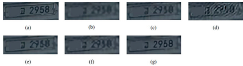
Figure 7. SR results of the second plate image (4×). (a) HR (140 × 48), (b) Bicubic, (c) DRN, (d) MZSR, (e) USRNet, (f) DBPN, (g) Proposed. Two characters were masked due to privacy policies.
