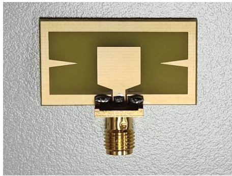
Figure 11. The prototype of the proposed antenna with an SMA connector soldered to it.
