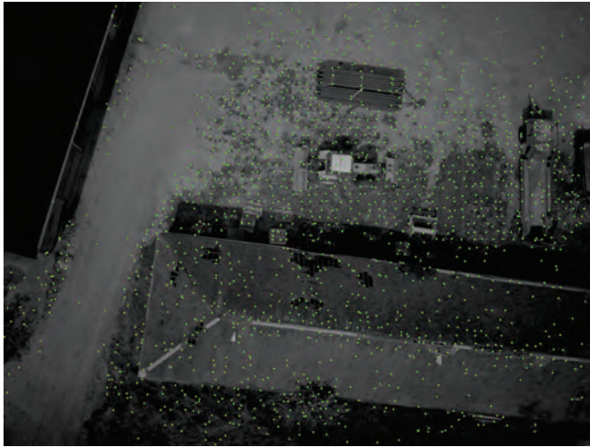
Figure 5. Uniform distribution of features over the image. The threshold intensity value of the detector is set to 7. This image is acquired with a low exposure time, but brightened artificially to clearly show the feature points. The size of the grid-adapted features is set to 100 \times 100 blocks.
