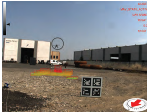
Figure 18. Simulated environment developed for the usability tests. The UAV is a 3D model simulated using the ArduCopter SITL simulator.
