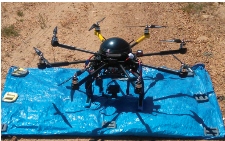
Figure 2. ATyges FV8 octocopter used for the aerial survey.
