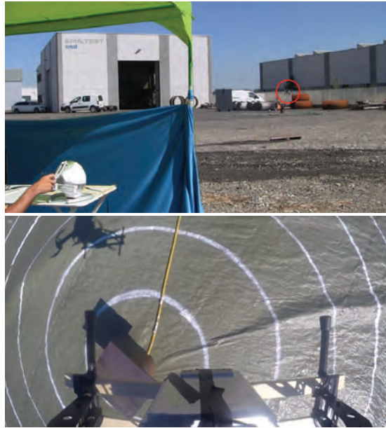
Figure 12. Detection of ^{192}\text{Ir} (located at the center of the target within the lead container) in a real environment using the position to position teleoperation mode. Experimental setup (top), where the UAV is highlighted by the red circle. Image taken from the onboard camera (bottom) when the operator affirmed that the current position of the UAV returned the maximum measured radiation. In this set of experiments, the gimbal unit was not used to get a clearer view of the ground from the onboard camera. The low speed of the UAV ensured that the gamma-ray detector remained parallel to the ground.
