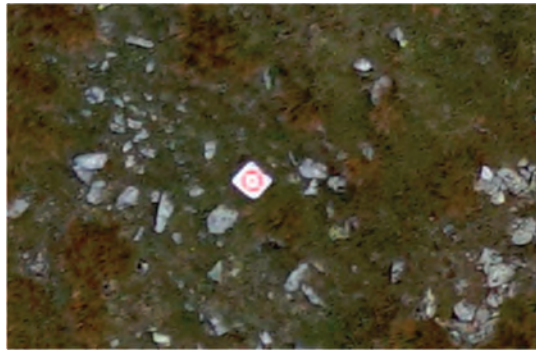
Figure 5. A control point on the image taken from the UAV (source: authors' own study).
