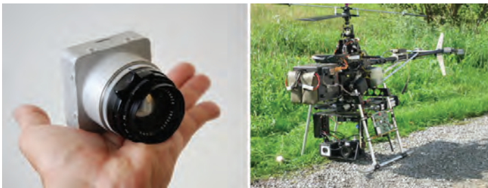
Figure 1. Institut national de l'information géographique (IGN) camera with the Copter 1B UAV developed by Wikydro.
