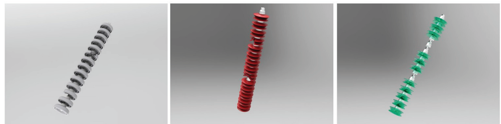
Figure 4. Artificial defect sample images of insulators (glass, ceramic and composite insulators).
