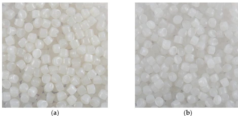
Figure 1. Images of the pellets of the virgin blow molding PE-HD grades vPE-1 (a) and vPE-2 (b).
