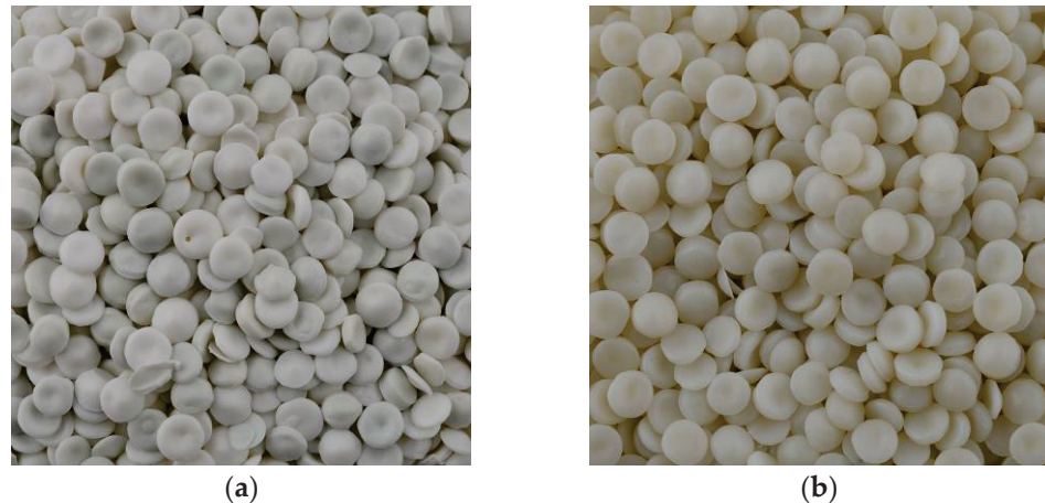
Figure 2. Images of the pellets of the PE-HD recyclates rPE-A in opaque white (a) and rPE-B in natural (b).
