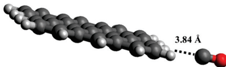
Figure 3. Computational simulation of the interaction between CO and graphene at 25 °C (carbon atoms were reported as black, oxygen atoms were reported as red and hydrogen ones as white). Reprinted with all permission from Dindorkar et al. [105].
