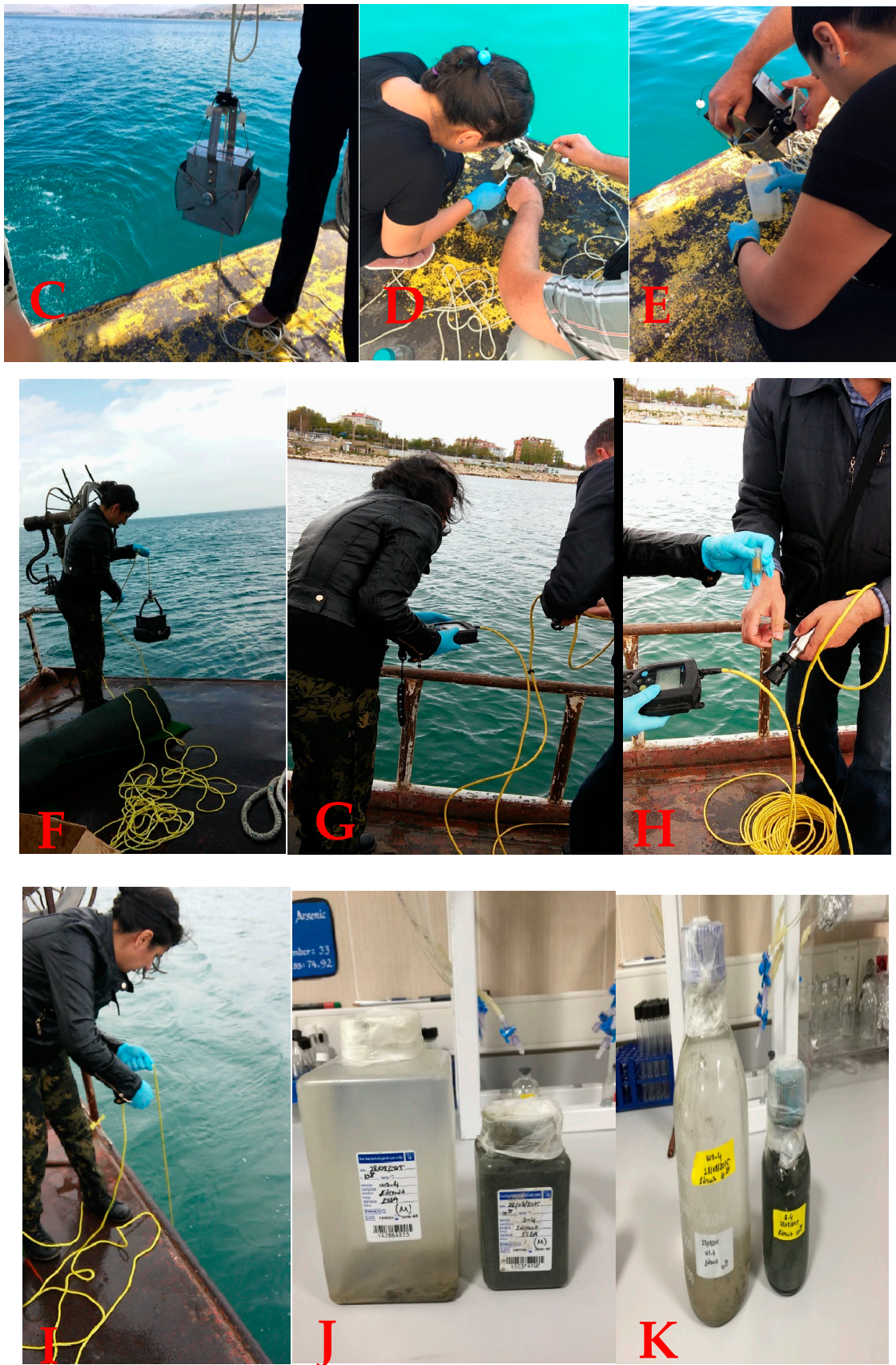
Figure A1. Pressure and salt resistant ladle (A–C) and sampling (D–K).
