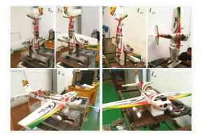
Figure 3. Characteristic Parameter Test.
