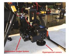
Figure 2. Assembly of the gimbal system and the Headwall Nano-Hyperspec<sup>®</sup> camera into the DJI S800 EVO unmanned aerial vehicle (UAV).
