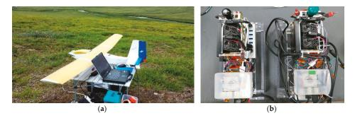
Figure 3. An example of the AggieAir "Minion" sUAS Fixed Wing Aircraft (a); and AggieAir custom payload detail (b).
