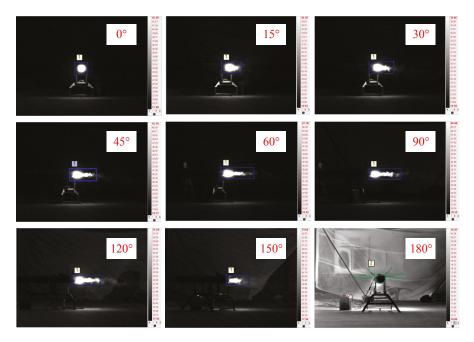
Figure 14. UAV images captured by the MWIR camera at different observation angles.
