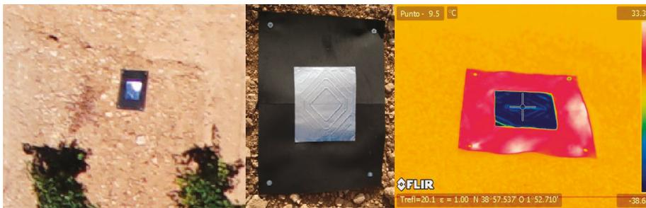
Figure 6. Type of GCPs used in thermal images.
