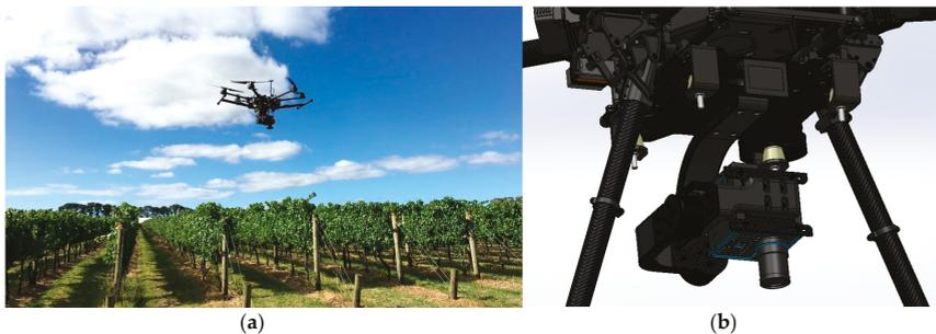
**Figure 5.** (a) Headwall Nano hyperspectral sensor on-board a S800 unmanned aerial vehicle (UAV); (b) Custom-made two-axis gimbal hosting the hyperspectral camera (SolidWorks 3D model).
